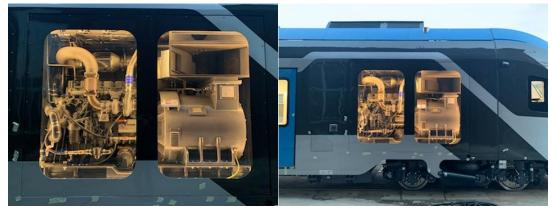
Fig. 3. Built-in powerpack generator in the type 227M rail vehicle [8]
