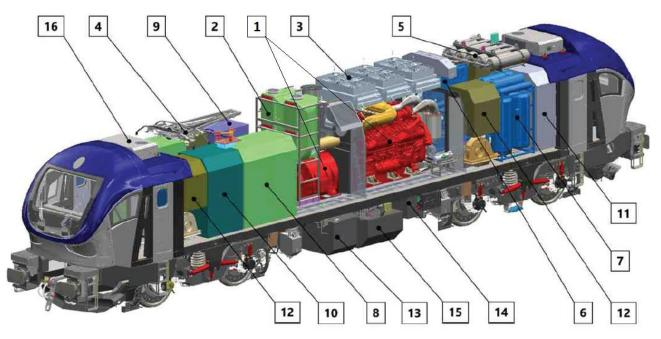
Fig. 4. Layout of equipment on the 111DE locomotive, 1 - power generator, 2 - a set of SCR catalytic systems, 3 - combustion engine cooling unit, 4 - pantograph, 5 - main air tanks, 6 - compressor module, 7 - board module, 8 - power inverters cabinet, 9 - cooling column with braking resistor, 10 - HV cabinet, 11 - ETCS cabinet, 12 - LV cabinet with electric motors ventilator, 13 - line choke, 14 - battery box, 15 - fuel tank, 16 - air conditioning unit [19]
