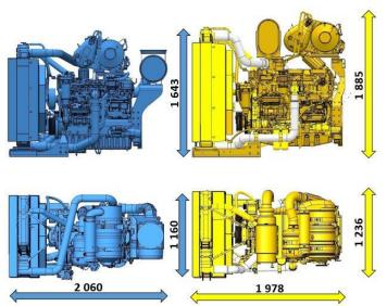
Fig. 11. List of internal combustion engines proposed for installation on the 501EH vehicle with dimensions provided. Top image shows the side view, bottom image shows the top view. Blue color CAT C9.3B engine, yellow color CAT C13B
