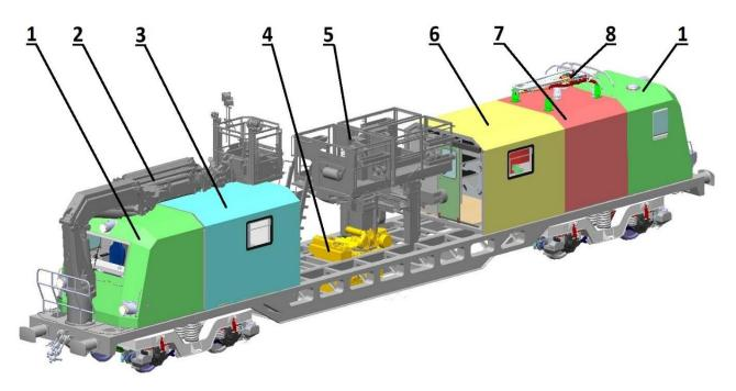
Fig. 9. The initial concept schematic of a 501EH special purpose vehicle;  $1 - driver's \ cabin$ ,  $2 - cherry \ picker \ basket \ and \ arm$ ,  $3 - crew \ rest \ compartment$ ,  $4 - combustion \ engine$ ,  $5 - cherry \ picker \ platform$ ,  $6 - workshop \ compartment$ ,  $7 - electrical \ module$ , 8 - pantograph
