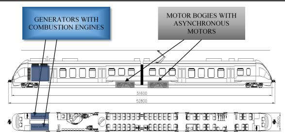
Fig. 2. Location of generating sets and motor bogies [8]
