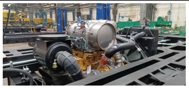
Fig. 12. An example of a CAT engine mounted in the free undercarriage space of a different type special purpose rail vehicle
